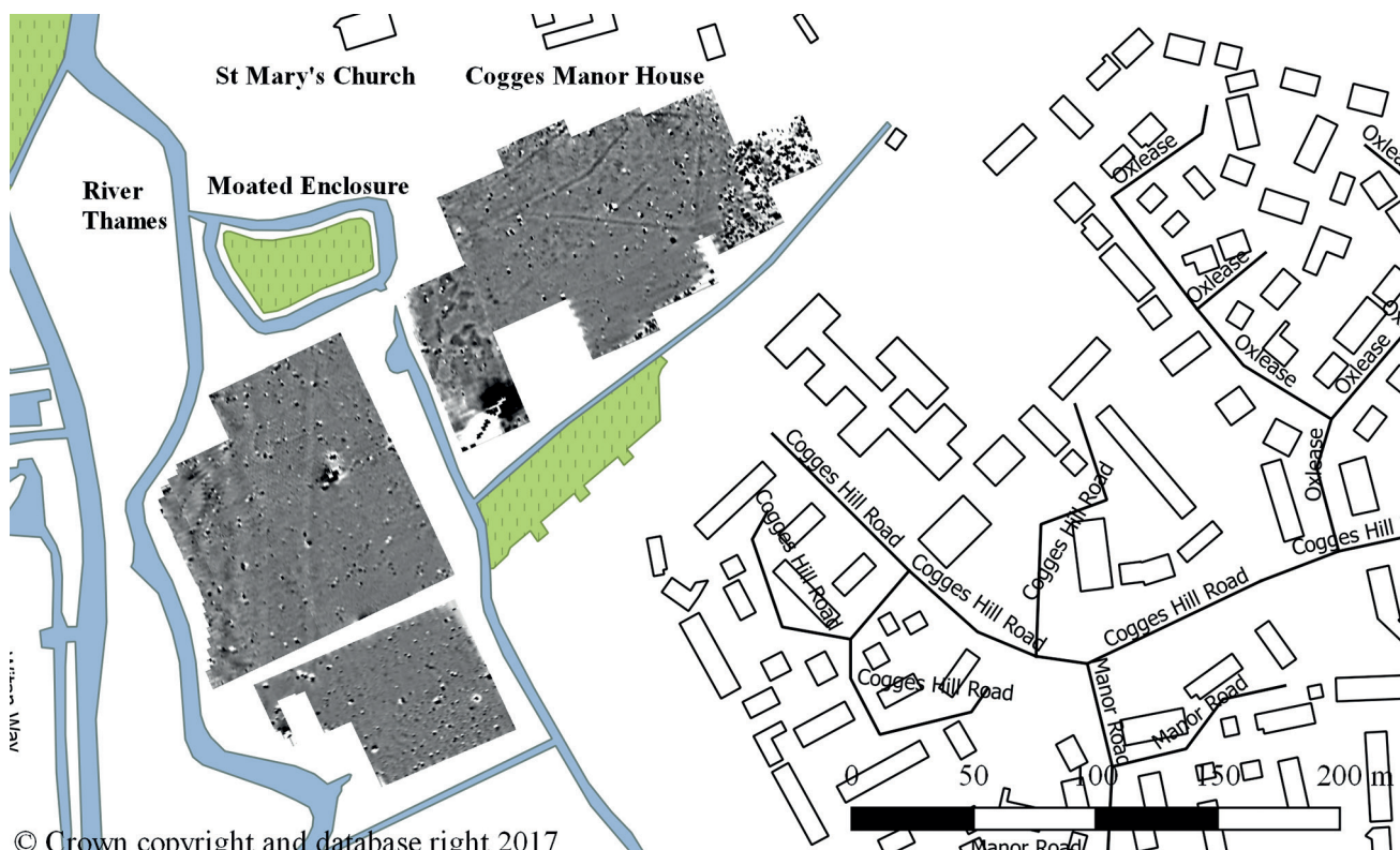
Figure 16: Magnetometer Surveys at Cogges Manor Farm, Witney, Oxfordshire
